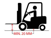
Keep a minimum ground clearance of 20 mm! (pay attention to the forks of a forklift truck!)
